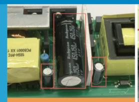
"PFC step-up output capacitor: The No.1 brand Rubycon from Japan is used, longer lifetime warranty."
