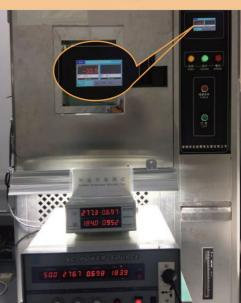
At as low as -30°C to -40°C, Tomcarline driver can still work properly at different working voltage
