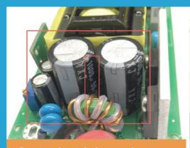
Output electrolytic capacitor: Rubycon brand with total output capacity 2000uF, ultra-Large capacity ensure longer lifetime.
