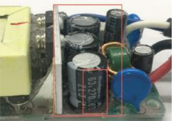
Output electrolytic capacitor: Rubycon brand with total output capacity 977uF, much less capacity cannot ensure long lifetime.
