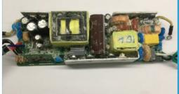
SMD and DIP components are mixed layout which interferes the driver performance; pouring sealant is low price polyurethane, high stress and serious pressing on components.
